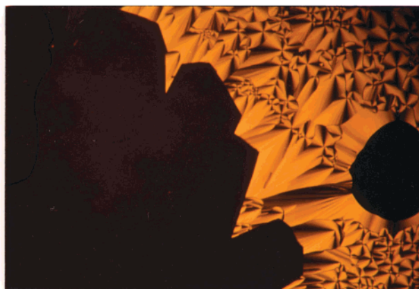
Figure 4. Micrographs showing the SmA-Cub phase transition for [\text{C15-Py}]_2[\text{CuCl}_4] as seen through crossed polarizers upon cooling from the smectic phase. From top to bottom: (top) nucleation of the cubic phase at 82 °C; (following plates) continued transition.
